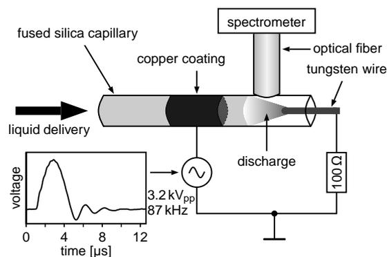
Fig. 1: Experimental arrangement of the LE-DBD
