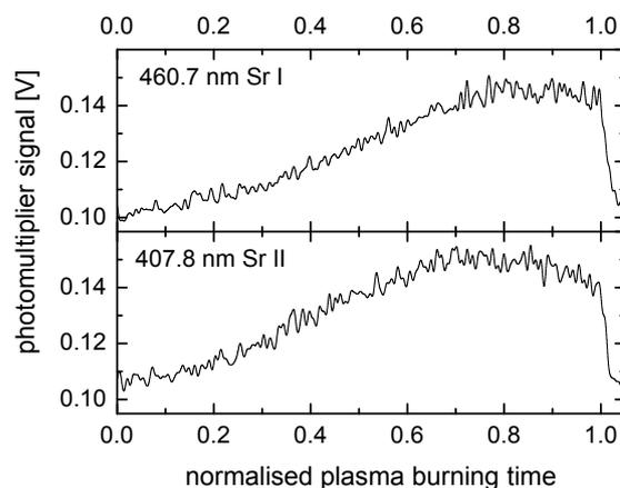
Fig. 5: Time development of the both strongest Sr emission lines during a plasma burning time.
