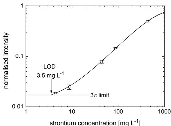
Fig. 4: Calibration curve for Sr in 1 mol L<sup>-1</sup> nitric acid using the 407,8 nm Sr II emission line.
