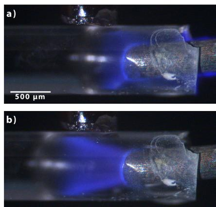
Fig. 2: Pulsation of the LE-DBD discharge. Picture a) shows the discharge after ignition where the trapezoid shape is not completely established and b) the plasma shortly before reaching its maximum size.
