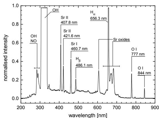
Fig. 3: Characteristic emission spectrum of 438 mg L<sup>-1</sup> Sr in 1 mol L<sup>-1</sup> nitric acid, measured with 100 ms integration time.
